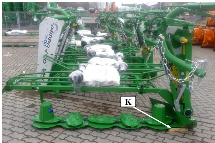
Fig. 22. Samba mower in vertical standstill position
